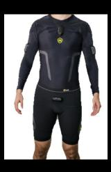
Smart wear collects data about physical loading of overall work physical load, during selected work phases, between different working techniques, or in comparing loading level of different tools or ergonomic solutions.
