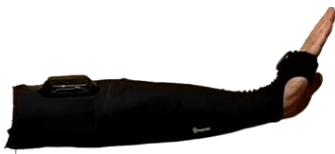
Fig 1. ErgoSleeve (Myontec, Finland) is an elastic smartwear with textile sensors in the inner layer of the product. Sensors measure wrist flexor and extensor muscle groups.
