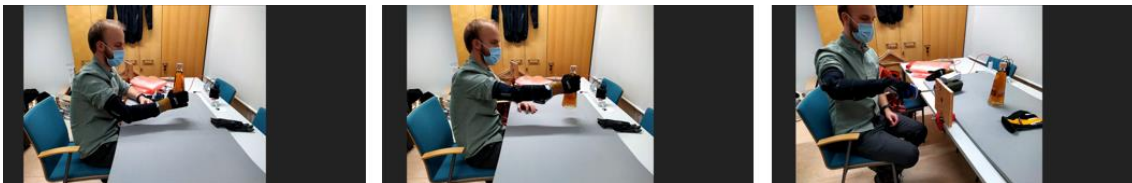
Figure 2. Testing movements consist of static grip to slow grip release (at wide position on left), (at narrow position on middle) and torsion movement with MicroClick torque screwdriver (on right).
